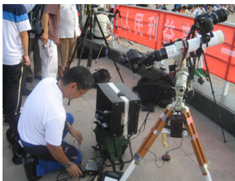
Jett making sure his equipment (video camera, still camera, and flash spectrum video), are all tracking, while connected to a laptop computer.
